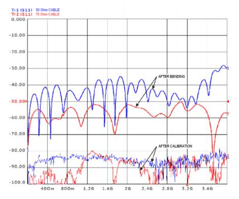
Using CMT Full-Size vector network analyzers with 50 $\Omega$  test ports, 5.7 dB MLP connected to the VNA test ports, and performing SOLT calibration with a high-quality calibration kit, we can expect the measurement error to be dependent only on the quality of the calibration kit, keeping impact of the 50 $\Omega$  to 75 $\Omega$  adapter to a minimum.
