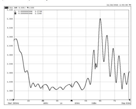
From the measurement results, we can see that the input VSWR, through the operating frequency, is always better than 1.4:1 and the transmission coefficient is about -6.4 dB for each output port. Therefore, our multiport testing system with RF switch is providing us a good measurement result that agrees with the datasheet.
