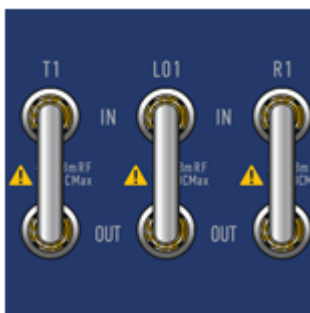
Location of connectors for the Frequency Extension Modules on the front and rear panels of the Cobalt C4220
