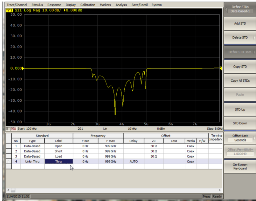
Figure 2: Create all the individual standards. Each databased standard should be specified as Type “Data-Based”.
